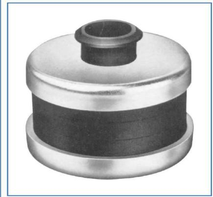
Style MUP Resilient Hanger consist of a resilient rubber mount held between two plated steel caps for uniform distribution of load.
