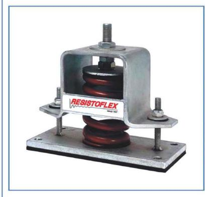
The ORS mounting has been designed specifically for applications where transmission of low frequency machinery vibration to a building structure must be reduced to avoid physical damage or annoyance to the the occupants. Vertical and lateral restraint is provided to control movement of the mounted equipment when subjected to external forces. This could otherwise be excessive due to the low stiffness springs required to provide isolation of low frequency vibration.
