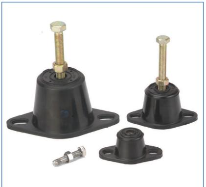
RM rubber mountings are designed to provide superior attenuation of medium to high frequency vibration and noise emanating from a wide range of motor driven machines particularly axial and centrifugal fans. High resillence rubber with low dynamic to static stiffness ratio ensures maximum efficiency, good creep performance and long service life.
