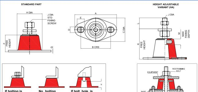
If bolting is preferred Mountings are furnished with a tapped hole in the centre. This enables the equipment to be bolted securely to the mounting.
