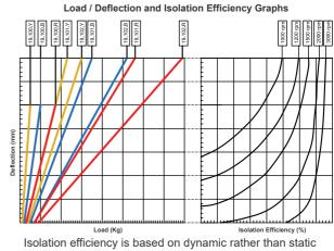
stiffness for accurate calculation of system performance.
